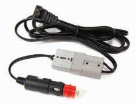
DC Power Cable (Can be Cigarette connection or Merit connection by removing/replacing red twist cap or Anderson plug connection by seperating the two anderson plug (Fig.4)
