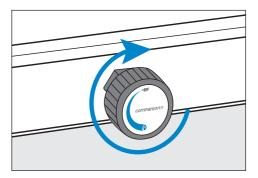
Turn the gas controls to the OFF position.
