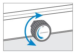
**Note:** When operating the appliance in windy conditions it is important to regularly check the burner to ensure that the flame has not been extinguished. If so turn the gas control off, allow residual gas to disperse. Relocate the appliance to a more sheltered position before attempting to reignite the burner.
