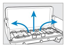
**Step 2.** Select the burner to be ignited and slowly turn the gas control in an anti-clockwise direction approximately ¼ of a turn.
