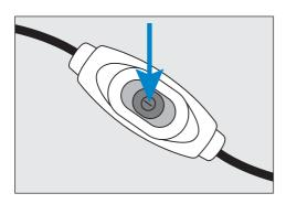
**Step 3.** Adjust flow of water as required using control on shower head.
