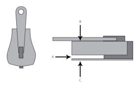
The most common reason why zips burst open is that the zip slider does not close the coil tightly enough. Metal fatigue and production variances cause the gap marked A to open up.
