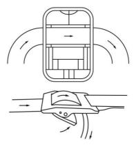
Position the camera and pull the loose end of the strap until the camera is firmly secured. To release the strap again, pull at the tab of the strap.
